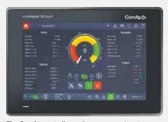
The ComAp controller and management system allows synchronisation of multiple generators on site, to bring in power only as it is needed. This leads to significant fuel savings each year.
