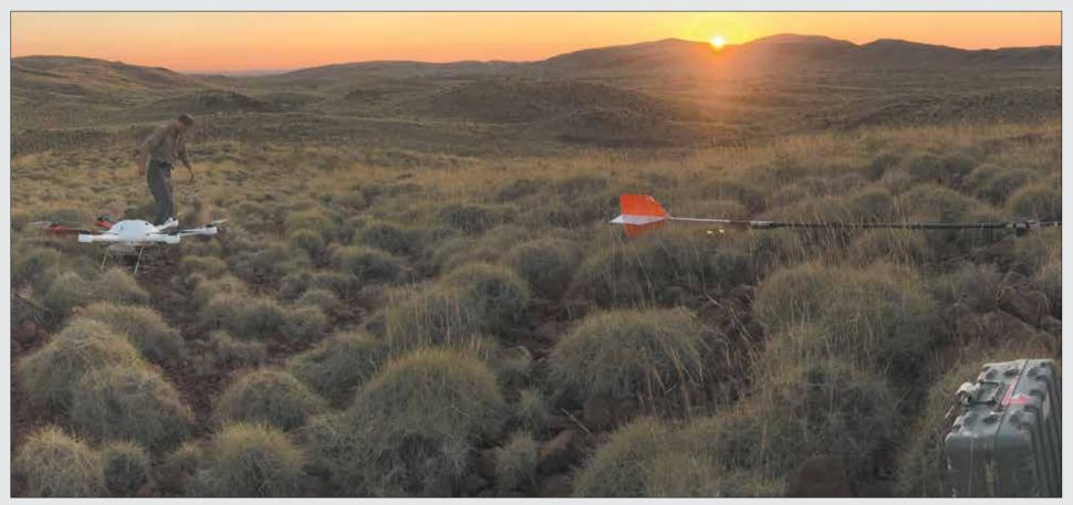
The custom-built hexacopter and magnetometer.
