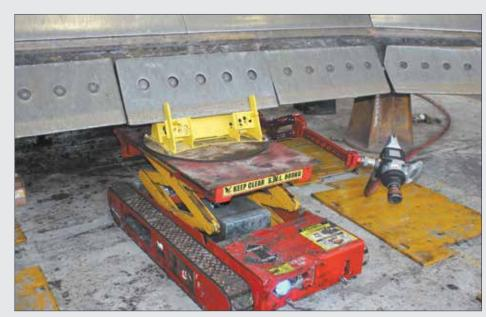
The TED is remote controlled - keeping fitters out of harm's way.
