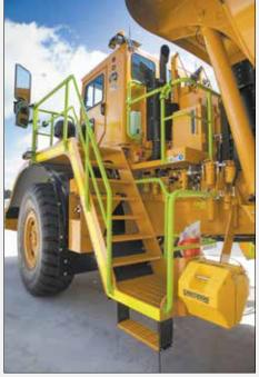
Stairs accessing the operator's cabin and the maintenance platform are bordered with safety rails allowing three points of contact.
