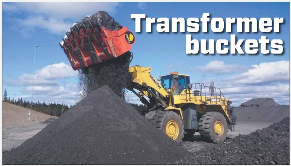
An ALLU M-Series processing bucket fitted to a Komatsu wheel loader.
