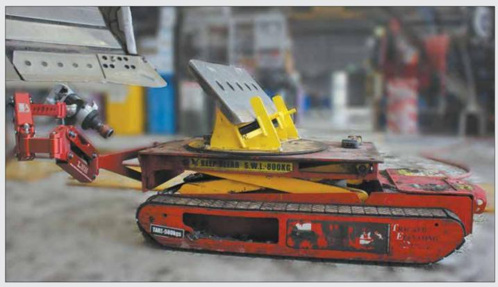
The tracked elevating device (TED) reduces manual handling and dramatically improves safety on site.
