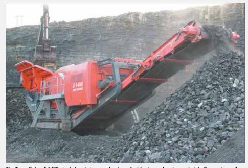
The Terex Finlay J-1480 single toggle jaw crusher is perfect for larger, tougher materials like coal, granite and limestone.
