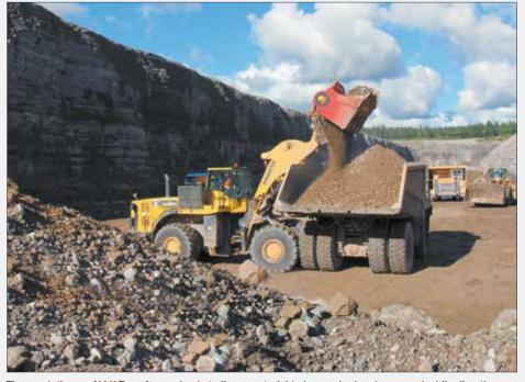
The revolutionary ALLU Transformer bucket allows material to be crushed and screened while directly loading haul trucks. This unique system brings the processing plant to the material for greater flexibility and substantial cost savings.
