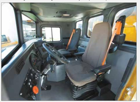
The spacious, ergonomically designed two-person ROPS / FOPS certified operators cabin offers a comfortable working space to minimise operator fatigue.
